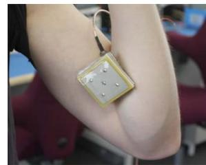
Fig. 11. Photograph of antenna in situ.
